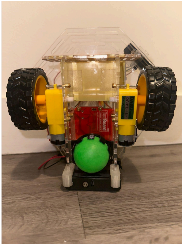
Photo of robot, highlighting the “airplane” wheel system
